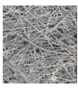
Each filter bag uses a prefilter to protect fine fibers from plugging. Media fiber distribution is carefully specified and controlled to deliver consistent, reliable high-efficiency filtration.
