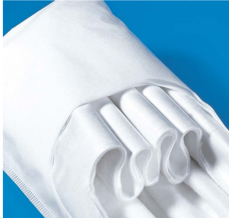
A pleated prefilter provides a very large surface (about 32 sq ft) to collect gels and solids before it reaches the final filter layers.
